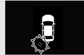
Example: Rear corner sensor (left) malfunctioning
